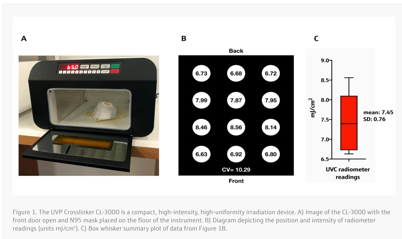
Figure 1. The UVP Crosslinker CL-3000 is a compact, high-intensity, high-uniformity irradiation device. A) Image of the CL-3000 with the front door open and N95 mask placed on the floor of the instrument. B) Diagram depicting the position and intensity of radiometer readings (units mJ/cm<sup>2</sup>). C) Box whisker summary plot of data from Figure 1B.
